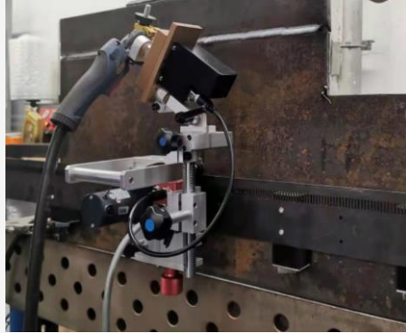
Transverse straight seam/circumferential weld welding
