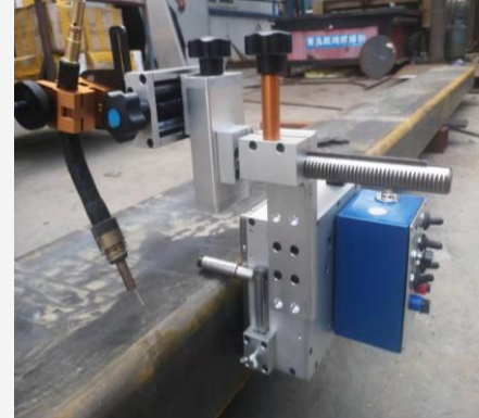
Box girder welding
