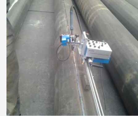
Longitudinal joint of pipe
