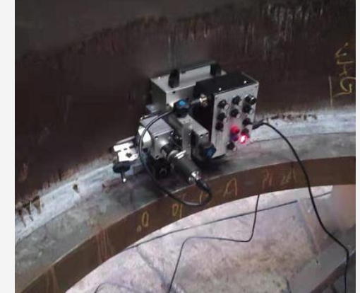
Suction-type oscillating fillet weld
