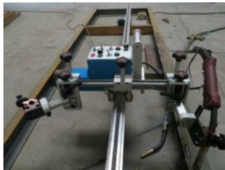
Straight seam double gun welding
